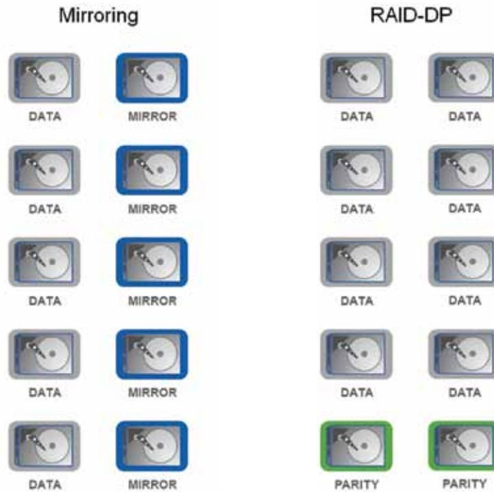
Figure 4) NetApp RAID-DP with double parity offers superior data protection compared to mirroring and up to 46% better storage efficiency.\*
